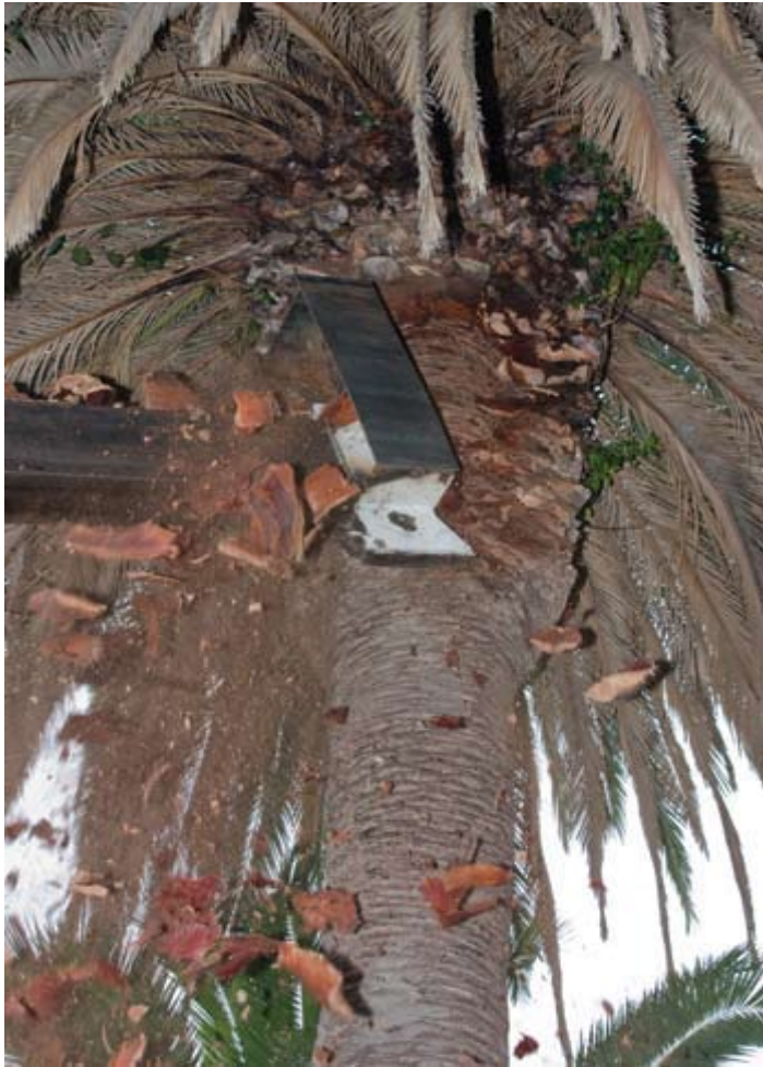
Figure 15. This innovative flange-like device, creatively mounted on the end of the hydraulic boom of a tower bucket truck and maneuvered by a skilled operator, has been effective in pushing off and shaping pineapples on Phoenix canariensis . Unlike a chain saw, it can be adequately disinfected to prevent disease spread.
